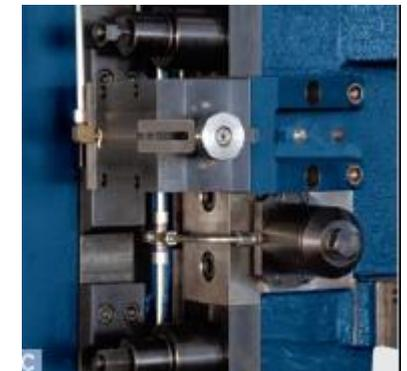
Double Column is programmable and clamp in place with pins.
