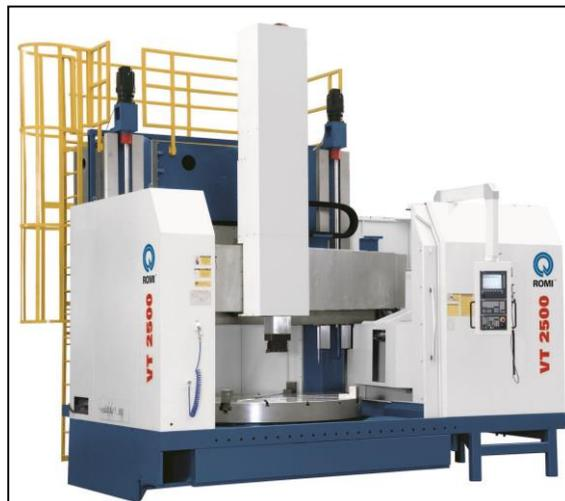
Headstock with 2 two continuously variable speed ranges, from: 1 to 51 rpm and 1 to 180 rpm, and 2700mm max cutting diameter, and 114hp / 84kW (regime 30min)
