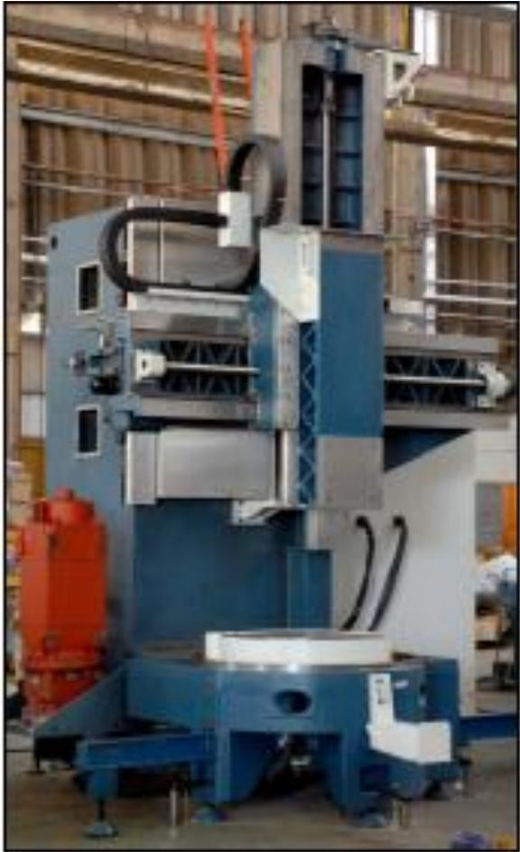
Column - The robust structure supports the cross rail and the vertical slide. The column is the basis for the machine rigidity, vibration absorbency and geometric stability. These are critical factors during heavy machining operations.
