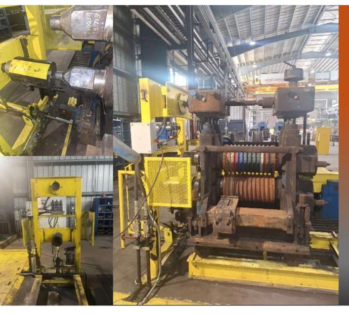
Alignment of the motors to the gearbox and spindles are critical. Remember not to make the coupling box rigid, it must float with the roll parting.
