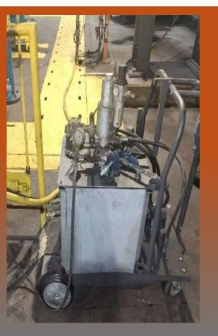
The Air/Oil unit is one of the most cost saving pieces of equipment to use. Verifying that the Air/Oil system is working the way it should eliminates the cost of downtime and replacing bearings and having chocks repaired or replaced.
