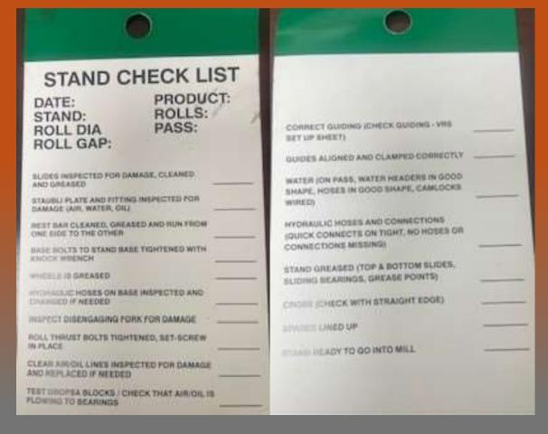
Prep work is so important and to verify that the work is audited we fill out our checklist and the stand is ready to go in the mill.
