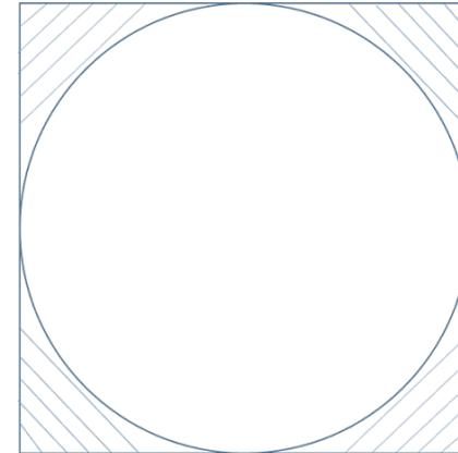
Area of cross-section of the beam = Shaded region
